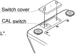
3. Press the CAL switch. The scale displays the "CAL".
